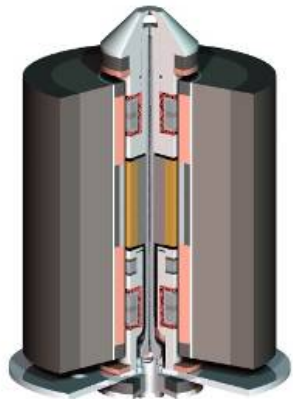
Flywheel system with Motor/Generator
