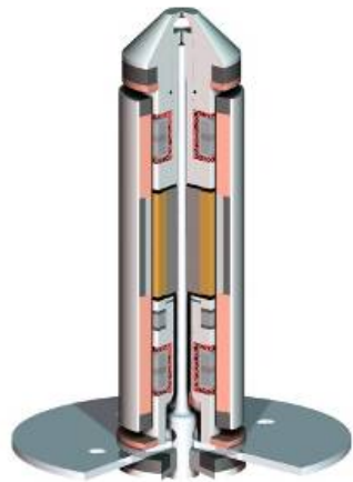
Magnetically levitated spindle unit with integrated drive
